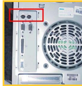
The keyboard and mouse ports sometimes look alike. In older computers, the mouse port may be larger, or square.
